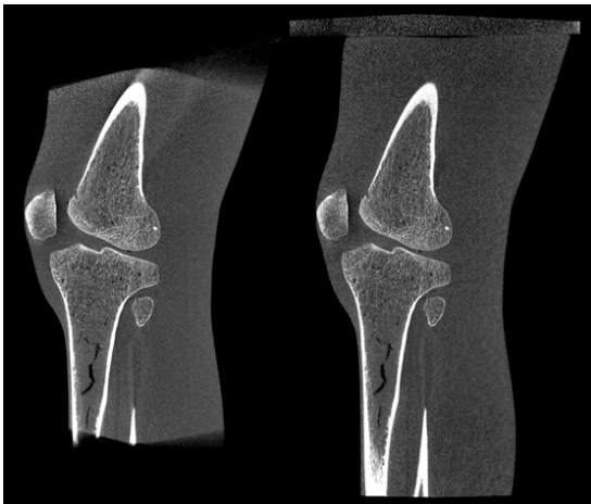
The image above demonstrates the additional Z-Axis reconstruction volume provided by the three-source configuration. (left image: single-source, right image: three-source).
