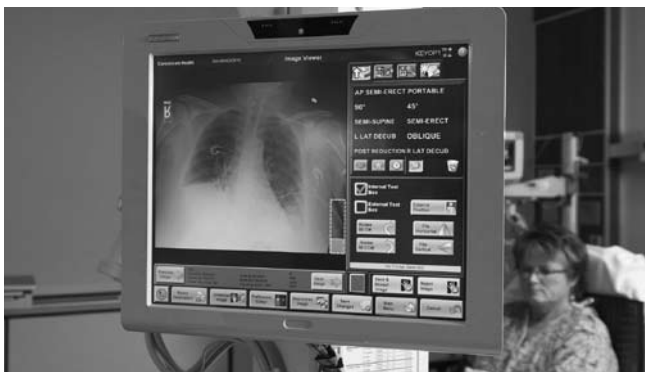
Heartland Regional Medical Center converted 5 existing mobile x-ray systems to DR with CARESTREAM DRX-Mobile Retrofit Kits. These mobile systems provide immediate image display on the monitor to enhance patient care in the ER, ICU and 10 operating suites.
